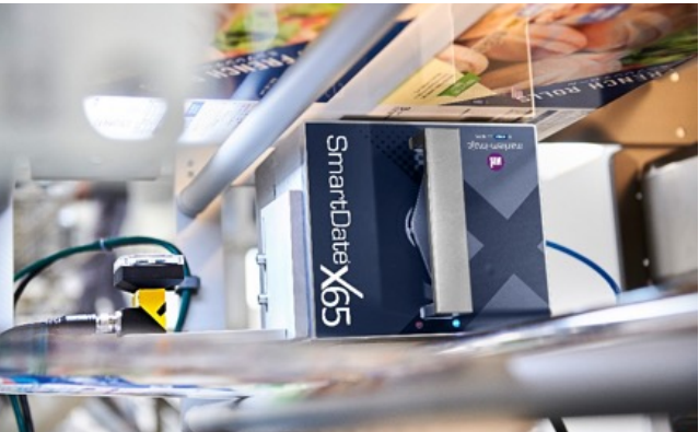
Markem-Imaje SmartDate® X65 thermal transfer coder is used to print on flexible film before filling
